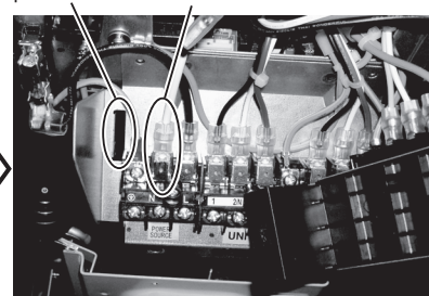
Square hole Disconnect the white cable
