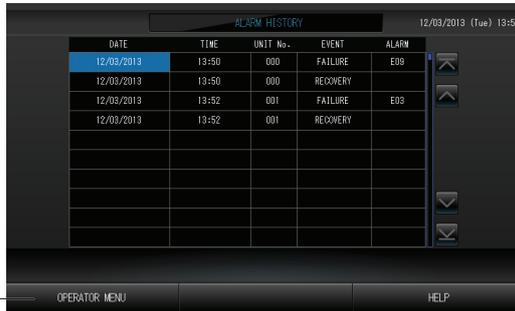
The screenshot shows the 'ALARM HISTORY' screen with a table of alarm events. The table has columns for DATE, TIME, UNIT No., EVENT, and ALARM. The data is as follows:
